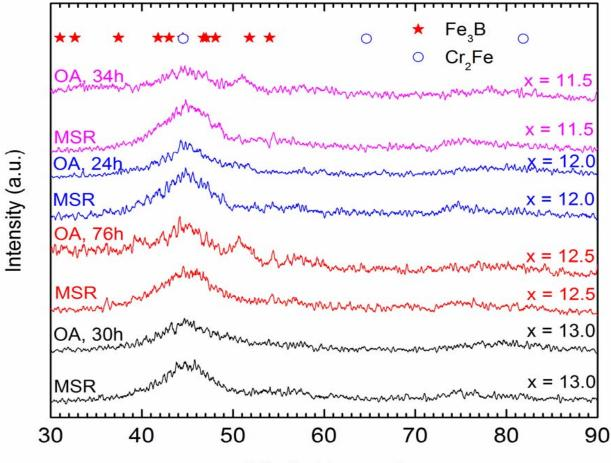
A glassy structure in the asquenched state, consisting of very weak magnetic Fe-Cr clusters (the inner part is rich in ferromagnetic Fe, whilst the outer shell is rich in antiferromagnetic Cr) surrounded by the Fe<sub>3</sub>Bbased residual matrix with enhanced  $T_c$  – the necessary condition to have low  $T_c$
