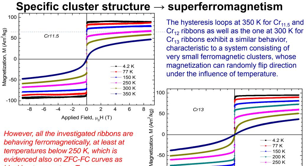
evidenced also on ZFC-FC curves as blocking temperature,  $T_b$ .
