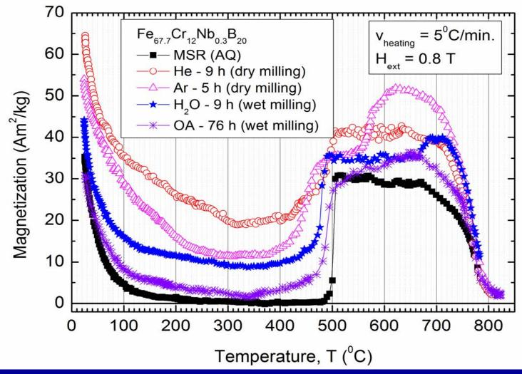
M(T) variation for  $Fe_{67.7}Cr_{12}Nb_{0.3}B_{20}$  glassy melt-spun ribbons and submicron powders milled in different conditions for different milling times. The transition temperature is strongly dependent on the microstructure of the milled submicron powders.
