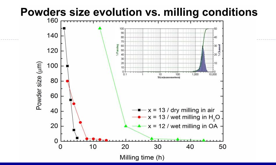
The dependence of size on milling conditions for  $Fe_{79.7-x}Cr_xNb_{0.3}B_{20}$  powders prepared by highenergy ball milling from glassy precursors. In the Inset is shown the size distribution of  $Fe_{67.7}Cr_{12}Nb_{0.3}B_{20}$  powders, milled in oleic acid for 44 h and determined by dynamic light scattering.
